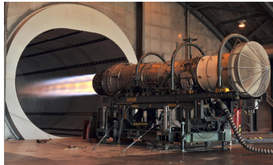
A Pratt & Whitney F100 turbofan engine for the F-15 Eagle being tested in the hush house at Florida Air National Guard base
